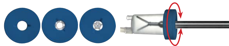
Rotary principle of the adapter seal
