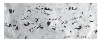
Foil after foil test in an ultrasonic bath with sonication from bottom and side
