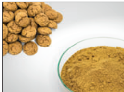
Cookies and vitamin tablets before and after comminution in the Knife Mill PULVERISETTE 11
